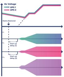
Dc voltage and AC current behaviour using the same value for delay time
