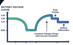
Normal Discharge EOD Charge with Temperature Protection Constant Voltage Compensation
